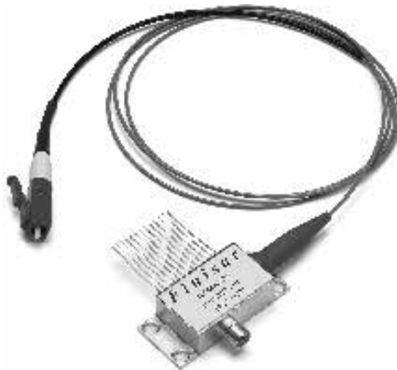
Fig. 4.42 An industry-standard laser diode mounted in a butterfly package. The fiber flylead is terminated with an LC optical connector. (Photo courtesy of Finisar Corporation; www.finisar.com .)
