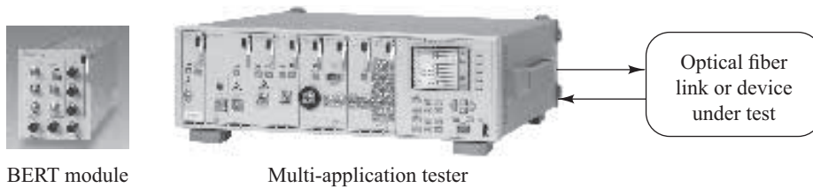
Fig. 14.32 A typical loopback BER test setup. (Photo courtesy of Yokogawa: Multi-Application Test System with BERT module; http://tmi.yokogawa.com .)
