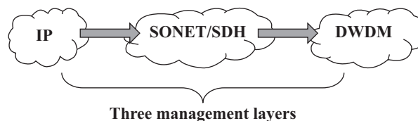
Fig. 13.49 Concept of an IP-over-SONET-over-DWDM architecture
