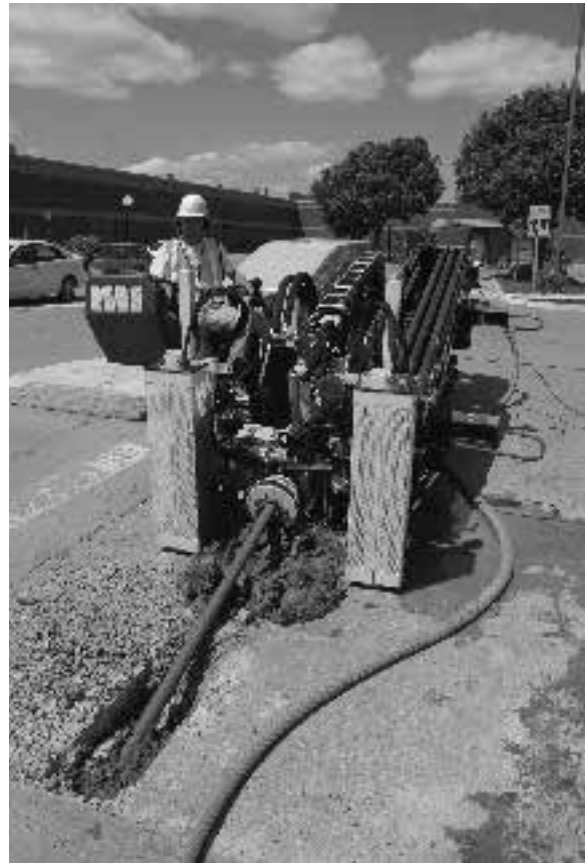
Fig. 2.48 Compact horizontal drilling machine for urban use. (Photo © VERMEER CORPORATION. All Rights Reserved; www.vermeer.com .)
