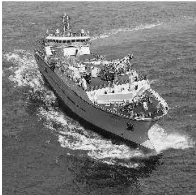
Fig. 1.13 Ship used to lay optical fiber cables across a sea or an ocean. (Photo courtesy of TE SubCom: www.SubCom.com .)
