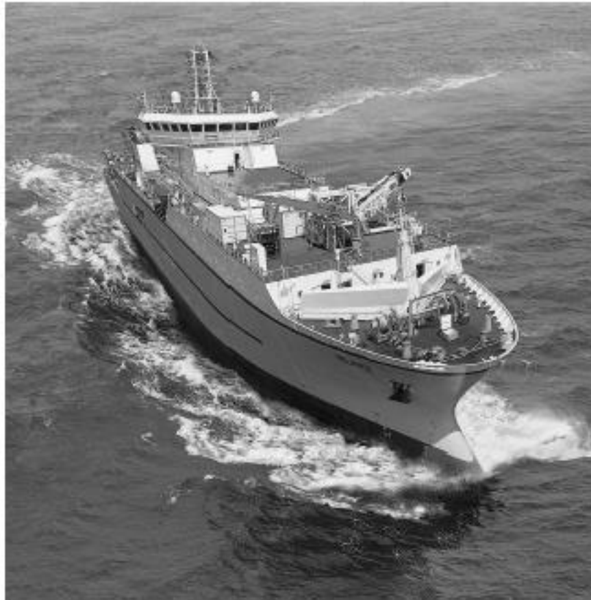
Ship used to lay optical fiber cables across a sea or an ocean. (Photo courtesy of TE SubCom: www.SubCom.com .)
